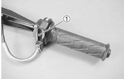
• Remove the throttle grip O from the tiller handle.
